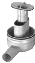
for construction heights from 95 mm, drainage capacity: 0.5 – 0.55 l/s*, water seal level: 50 mm (can be shortened to reconstruction model) Model 4982.92
