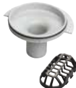
vertical model without: odour trap Drainage capacity accumulation height 10 mm 1.2 l/s Drainage capacity accumulation height 20 mm 1.2 l/s Model 4982.83
