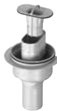
vertical model for construction heights from 40 mm, drainage capacity: 0.9 – 1.1 l/s*, water seal level: 50 mm (fire protection pipe lead-in possible) Model 4982.94
