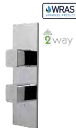
THERMO VALVE 2 OUTLET Recessed 2 way diverter Minimum pressure 1bar HP H:180mm W:60mm
